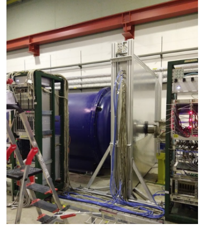
Figure 4.2: Left: A schematic of the ANTI-0 detector showing the support frame, central sheet and counters. Note the horizontal line just below the mid-point of the detector delimiting the top and bottom parts. [101] Right: Picture of the ANTI-0 as installed in TCC8, with the blue decay vessel to the left and beam pipe to the right. [107]
