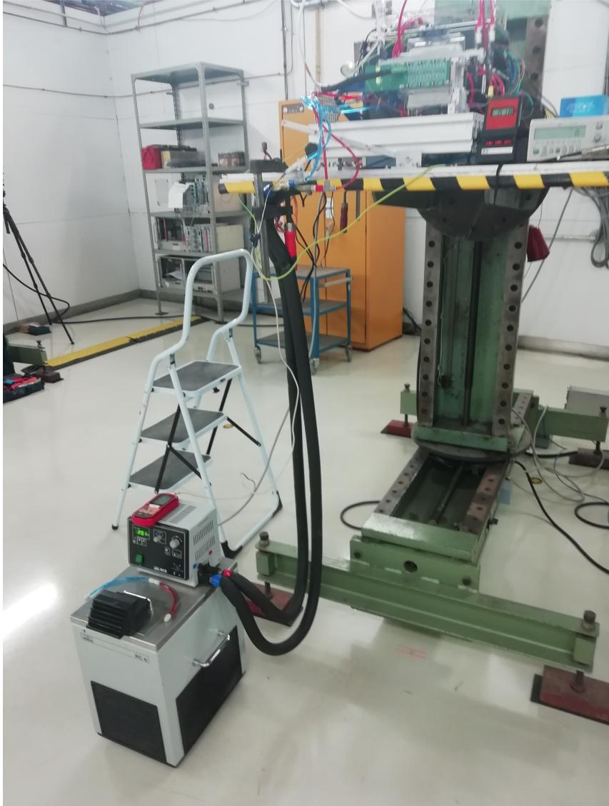
Figure 6.15: The water-cooling system used to maintain a steady temperature over the EPICAL-2 prototype during data-taking in February 2020.
