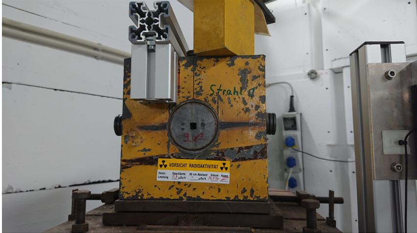
Figure 6.12: Secondary collimator used in the test beam areas TB24/1 at DESY II.
