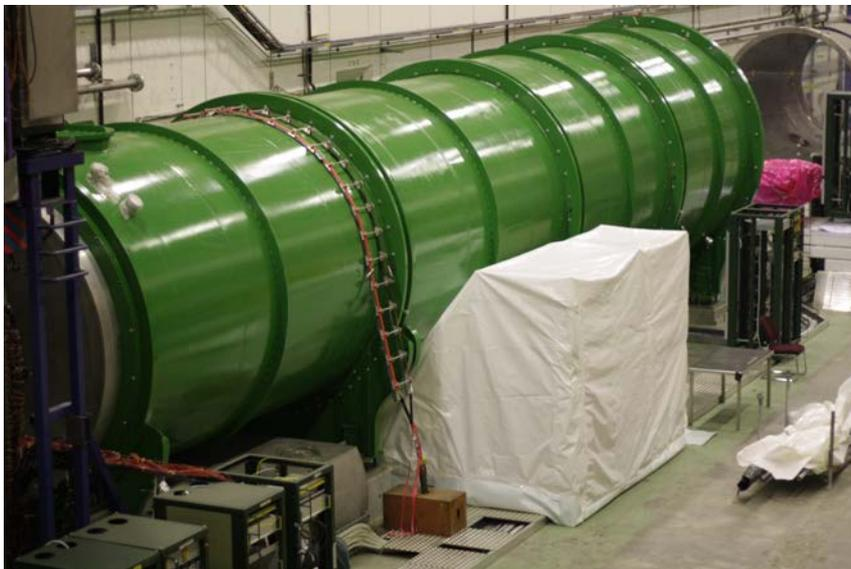
Figure 4.10: The RICH vessel installed in the NA62 cavern.
