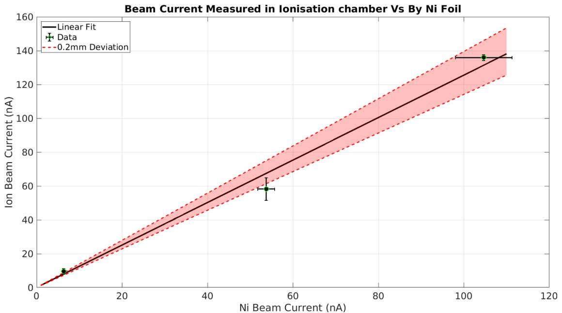
Figure 7.16: Beam current measured via ionisation chamber vs via nickel foil, including a 0.2 mm deviation in the ionisation chamber gap width.
