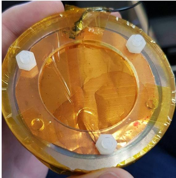
Figure 7.10: Ionisation chamber top down.
