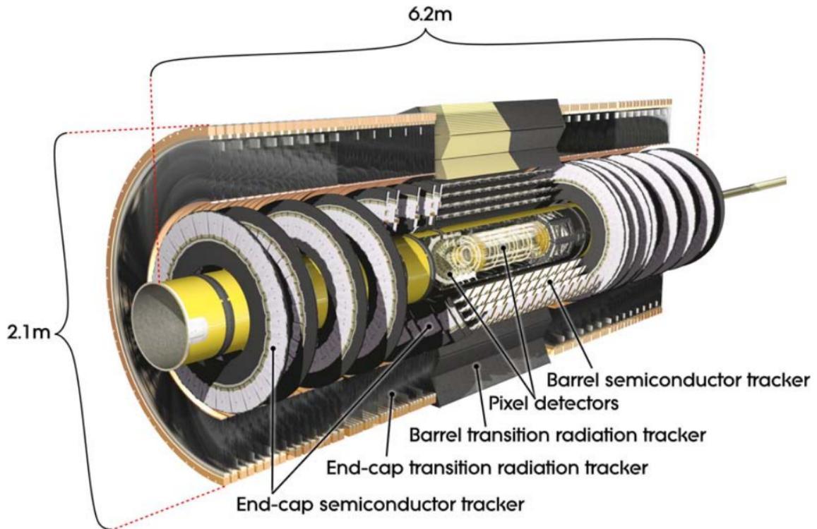
Figure 3.9: Cut-away view of the ATLAS Inner Detector [47].
