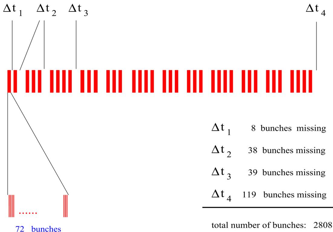
Figure 3.2: An example filling scheme, showing all the buckets in a fill, buckets which are filled with proton bunches are shown in red. There is a long gap ( $\Delta t_4$ ) after the final filled bunch before repeating to help with beamdumps. [43].
