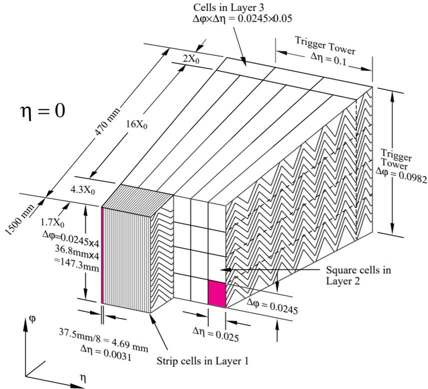
Figure 3.12: The electromagnetic calorimeter accordion geometry, showing all three layers. Only layer 2 and layer 3 are present above  $|\eta| = 2.5$ . An individual section, highlighted in pink, is called a cell [45].
