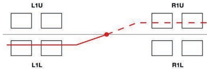
Figure 7.3: A simplified elastic interaction demonstrating the tag and probe method used for ALFA reconstruction efficiency calculations. L1L is identified as the ‘tag’ and the R1U armlet is ‘probed’.
