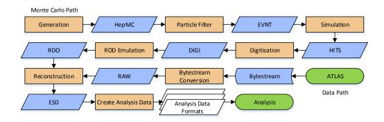
Figure 7.1: The flow of ATLAS data from event generators and through the simulation software or from the detector with both routes passing through to reconstruction and analysis.
