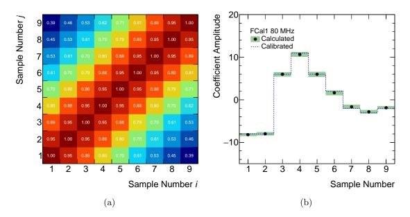
Figure 6.9: Calibration of filter coefficients for a trigger tower in the EMEC IW with 80 MHz sampling and 25 ns bunch spacing. (a) shows the correlation matrix  $\boldsymbol{R}$  between samples and (b) shows the corresponding filter coefficients  $\boldsymbol{a}$  after normalisation.
