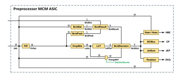
Figure 5.3: Overview of Preprocessor MCM ASIC logic for one channel. The ADC data enters the processing logic from the left-hand side and the results are sent on to the systems marked on the right-hand side.
