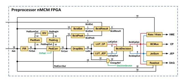
Figure 6.11: Overview of Preprocessor nMCM FPGA logic for one channel that includes both the MCM logic shown in Figure 5.3 and processing blocks for the pedestal correction and additional LUT.
