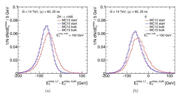
Figure 7.15: Distributions of the difference between the Level 1 and Topo  $E_{\rm T}^{\rm miss}$  for (a)  $ZH \rightarrow \nu \bar{\nu} b \bar{b}$  events and (b)  $t\bar{t}$  events in the MC12 and MC15 simulation with  $E_{\rm T}^{\rm miss, \ truth} > 100 \,{\rm GeV}$  and separated by the position in the bunch train.
