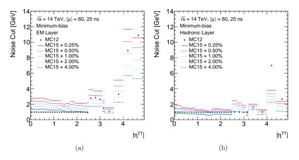
Figure 7.3: Noise cut thresholds in GeV as a function of the trigger tower  $|\eta|$  for (a) the EM and (b) hadronic calorimeter layers for MC12 and different occupancy values in MC15.
