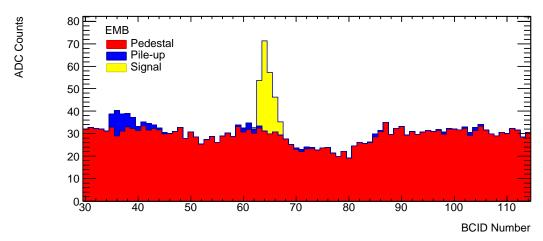
(a) ADC input into the FIR Filter
