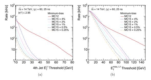
Figure 7.4: Level 1 trigger rate as a function of the  $E_{\rm T}$  threshold for (a) four-jet and (b)  $E_{\rm T}^{\rm miss}$  triggers in MC12 and MC15 with different noise cut configurations.
