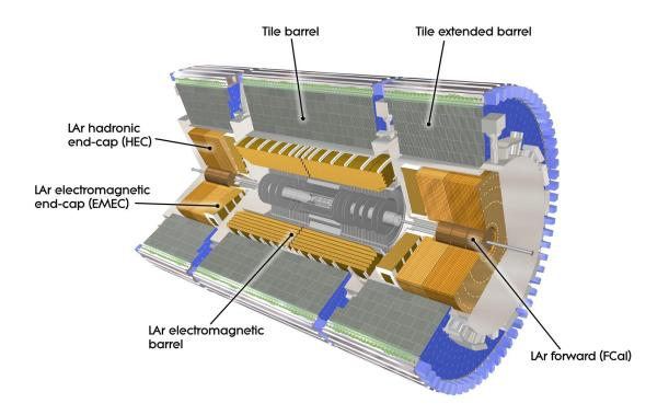
Figure 4.3: Overview of the ATLAS calorimetry systems. ©CERN.
