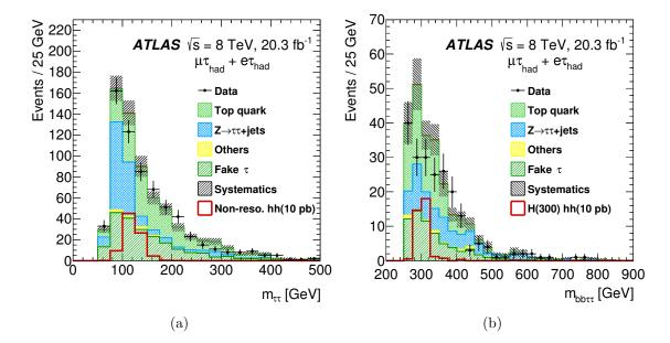
Figure 8.11: Distributions of final discriminants combining all analysis categories: (a)  $m_{\tau\tau}^{\text{MMC}}$  for the nonresonant search and (b)  $m_{bb\tau\tau}$  for the resonant search. The single SM Higgs boson background is too small to be seen and the nonresonant signal distribution is shown assuming a cross section of 10 pb for Higgs boson pair production.
