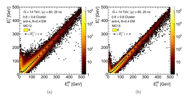
Figure 7.8: Correlation between Level 1 and anti- $k_t R = 0.4$  EM-scale jets in  $t\bar{t}$  events for (a) MC12 and (b) MC15 simulations. The overlaid data points and vertical error bars represent the mean and standard deviation of the distributions of Level 1 jet  $E_{\rm T}$ , respectively.
