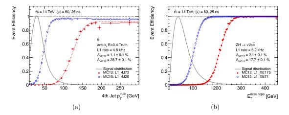
Figure 7.5: Level 1 event efficiency turn-on curves for (a) four-jet triggers in  $t\bar{t}$  events and (b)  $E_{\rm T}^{\rm miss}$  triggers in  $ZH \rightarrow \nu \bar{\nu} b\bar{b}$  events. The trigger thresholds indicated in the legends have been selected for the same trigger rate in the MC12 and MC15 simulations.
