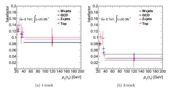
Figure 8.8: Fake factors for the W + jets, QCD, Z + jets and top control regions as a function of the hadronic tau candidate  $p_{\rm T}$ . The error bars show the statistical uncertainty only.
