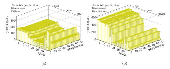
Figure 7.2: Average FIR output of the autocorrelation filters in minimum-bias simulated events per  $|\eta|$ -bin and over one bunch train for trigger towers in (a) the EM and (b) hadronic calorimeter layers.
