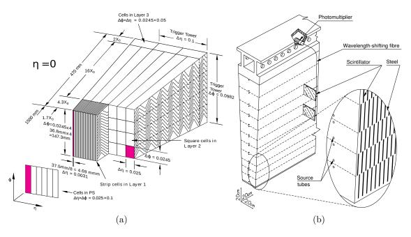
Figure 4.4: Schematic view of (a) the LAr accordion structure and (b) a single Tile module or 'drawer' [27].
