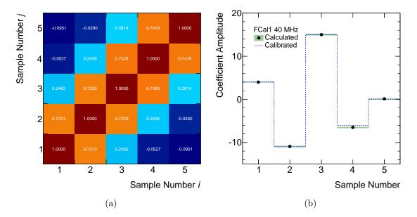
Figure 6.7: Calibration of filter coefficients for a trigger tower in FCal1 with 40 MHz sampling and 25 ns bunch spacing. (a) shows the correlation matrix  $\boldsymbol{R}$  between samples and (b) shows the corresponding filter coefficients  $\boldsymbol{a}$  after normalisation.
