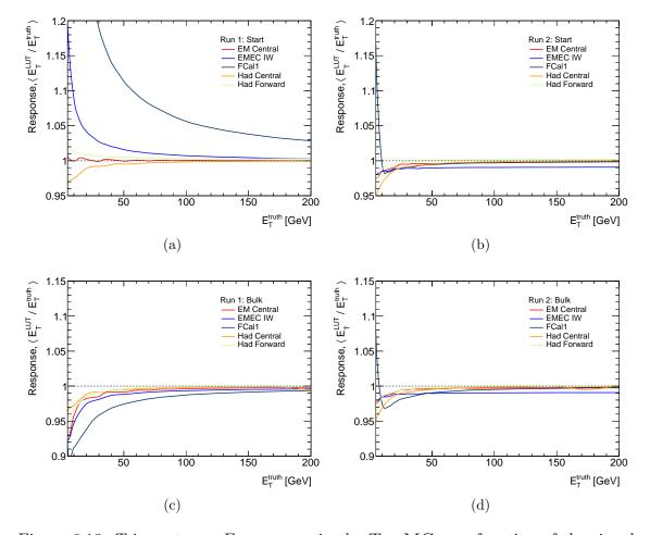
Figure 6.13: Trigger tower  $E_{\rm T}$  response in the TOYMC as a function of the signal pulse  $E_{\rm T}$  in different calorimeter regions. Subfigures (a) and (b) are for the Run 1 and Run 2 configurations at the start of the bunch train. Subfigures (c) and (d) are for the Run 1 and Run 2 configurations in the bulk of the bunch train.
