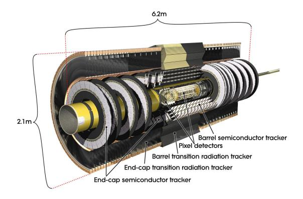
Figure 4.2: Cut-away view of the ATLAS inner detector. ©CERN.
