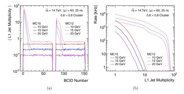
Figure 7.6: Level 1 jet multiplicities passing different thresholds in the MC12 and MC15 simulation for minimum-bias events. Subfigure (a) shows the average number of Level 1 jets as a function of the BCID number for a bunch train proceeding a long and short gap. Subfigure (b) shows the inclusive rate at which Level 1 jet multiplicities are satisfied.
