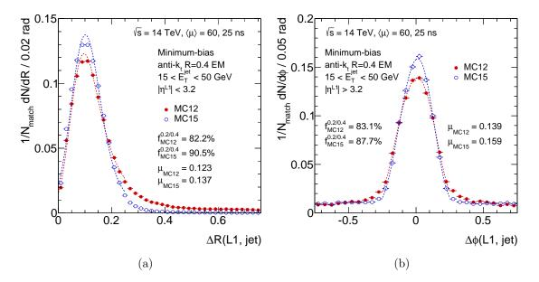
Figure 7.7: Closest distance between Level 1 and calorimeter jets with  $15 < E_{\rm T}^{\rm jet} < 50 \,{\rm GeV}$ , normalised to the number of matched jets for MC12 and MC15, using minimum-bias events. The  $\Delta R$  for Level 1 RoIs outside FCal is shown in (a), while (b) shows the  $\Delta \phi$  for Level 1 RoIs within FCal.
