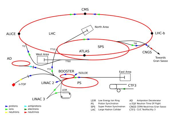
Figure 3.2: Schematic diagram of the CERN accelerator complex. Derived from [75].
