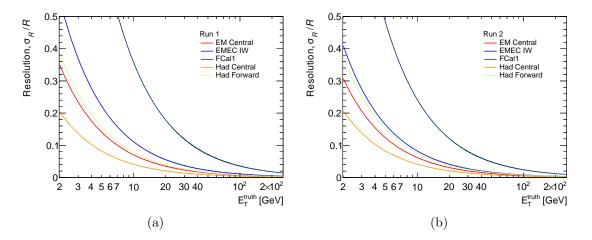
Figure 6.14: Fractional trigger tower  $E_{\rm T}$  resolution in the TOYMC as a function of the signal pulse  $E_{\rm T}$  for different calorimeter regions for the (a) Run 1 and (b) Run 2 configurations.
