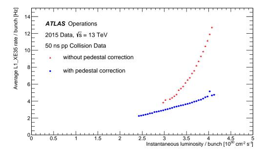
Figure 7.20: Level 1 trigger rate per bunch as a function of the instantaneous luminosity per bunch for the  $E_{\rm T}^{\rm miss}$  trigger with a 35 GeV threshold [124]. The rates are shown with and without the pedestal correction applied.
