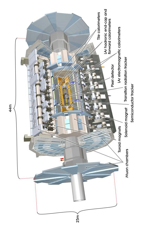
Figure 4.1: Cut-away view of the ATLAS detector. ©CERN.
