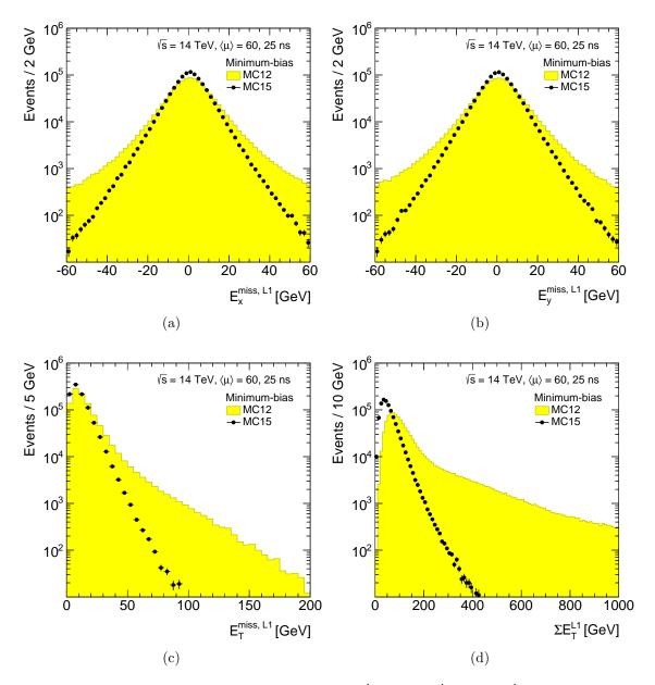
Figure 7.13: Distributions of the Level 1 (a)  $E_x^{\text{miss}}$ , (b)  $E_y^{\text{miss}}$ , (c)  $E_T^{\text{miss}}$  and (d)  $\sum E_T$  as measured in minimum-bias events for the MC12 and MC15 simulations.
