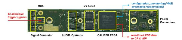
Figure 5.9: The topside view of the new Preprocessor MCM. The four analogue trigger tower signals enter the module on the left-hand side and are digitised by the dual ADCs before entering the FPGA, where the main processing occurs. Taken from [85].
