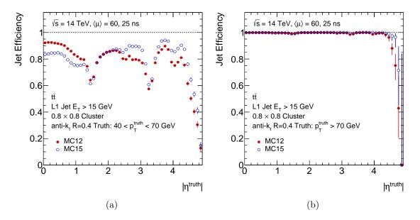
Figure 7.12: The efficiency in MC12 and MC15 for anti- $k_t R = 0.4$  truth jets in  $t\bar{t}$  events to satisfy a Level 1 threshold of 15 GeV as a function of the truth jet  $|\eta|$  for (a)  $40 < p_T^{\text{truth}} < 70 \text{ GeV}$  and (b)  $p_T^{\text{truth}} > 70 \text{ GeV}$ .
