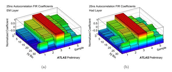
Figure 7.18: Normalised autocorrelation FIR filter coefficients for a 25 ns bunch spacing for each  $|\eta|$ -bin in (a) the EM layer and (b) the hadronic layer [124].
