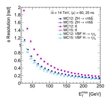
Figure 7.16: Azimuthal resolution of the  $E_{\rm T}^{\rm miss}$  vector as a function of the true  $E_{\rm T}^{\rm miss}$ in MC12 and MC15 for three different physics processes:  $ZH \rightarrow \nu \bar{\nu} b \bar{b}$ , semi-leptonic  $t\bar{t}$  and VBF  $H \rightarrow \tau_{\ell} \tau_{h}$  events. The data points for each process have different offsets with respect to the bin centre for clarity.
