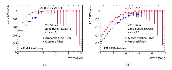
Figure 7.19: The efficiency that a calorimeter pulse is identified in the correct bunch crossing as a function of the offline  $E_{\rm T}$  [124]. The performance of the matched filter is compared to the autocorrelation filter for (a) the EMEC IW and (b) FCal1.
