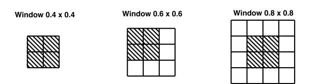
Figure 5.7: Jet trigger algorithm operates on jet elements indicated by the  $0.2 \times 0.2$  grid. The three available  $E_{\rm T}$  cluster sizes of  $2 \times 2$ ,  $3 \times 3$  and  $4 \times 4$  jet elements are shown with the corresponding RoIs given by the shaded regions. Taken from [76].
