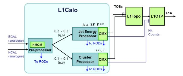
Figure 5.8: Overview of the L1Calo system architecture during Run 2. Pre-exisiting components are shown in blue and the new components are shown in green. Taken from [85].
