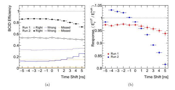
Figure 6.15: FCall performance comparison in the ToYMC between the Run 1 and Run 2 configurations for systematic timing shifts from -5 ns to +5 ns. Subfigure (a) shows the BCID efficiency for 5 GeV signals. The black points show correctly identified signals, the blue lines show where the peak-finder fires one bunch crossing early or late, and the yellow lines show the signals missed by the peak-finder. Subfigure (b) shows the response for 30 GeV signals.
