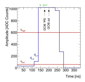
Figure 5.5: Illustration of the BCID algorithm for saturated signals. The two ADC values  $d_{s-2}$  and  $d_{s-1}$  are compared to the programmable thresholds  $s_{\text{low}}$  and  $s_{\text{high}}$  to determine if the correct bunch crossing is s or s + 1. In this case, the peak-finder BCID fires one bunch crossing late.
