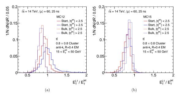
Figure 7.9: Response distributions between Level 1 and  $\operatorname{anti-}k_t R = 0.4$  EM-scale jets with  $15 < E_{\mathrm{T}}^{\mathrm{jet}} < 50 \,\mathrm{GeV}$  for (a) MC12 and (b) MC15 using  $t\bar{t}$  data. The distributions are separated by the position in the bunch train and for  $|\eta| < 2.5$  and  $|\eta| > 2.5$ .
