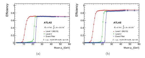
Figure 4.8: Single muon trigger efficiencies after the L1, L2 and EF selections as a function of offline reconstructed muons for (a) the barrel region and (b) the endcap region. The efficiencies were measured with a tag-and-probe method using  $Z \rightarrow \mu\mu$  decays for the mu24i\_tight OR mu36\_tight trigger and are shown with statistical uncertainties [90].
