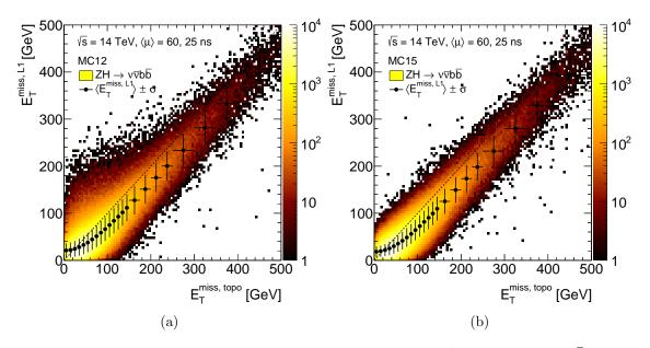
Figure 7.14: Correlation between the Level 1 and Topo  $E_{\rm T}^{\rm miss}$  for  $ZH \rightarrow \nu \bar{\nu} b \bar{b}$  events in (a) the MC12 and (b) the MC15 simulations. The overlaid data points and vertical error bars represent the mean and standard deviation of the distributions of Level 1  $E_{\rm T}^{\rm miss}$ , respectively.
