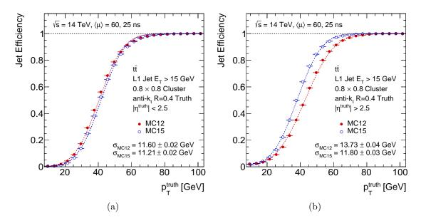
Figure 7.11: The efficiency in MC12 and MC15 for anti- $k_t R = 0.4$  truth jets in  $t\bar{t}$  events to satisfy a Level 1 threshold of 15 GeV as a function of the truth jet  $p_{\rm T}$ , integrating over (a)  $|\eta| < 2.5$  and (b)  $|\eta| > 2.5$ . Only events occurring in later bunches in a train are used.
