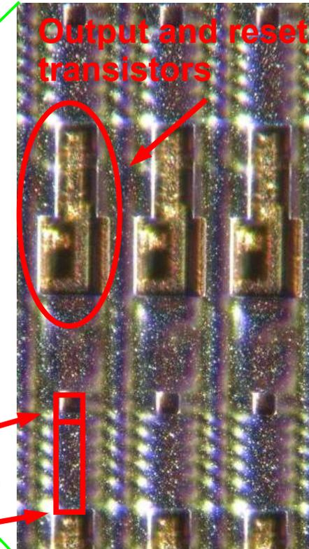
Photogate aperture (8  $\mu\text{m}$  square)
