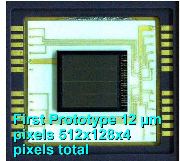
Layout of prototype ASIC
