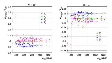
Loop contributions to  $H \to gg$  (left) and  $\gamma\gamma$  (right) in 4DCHM normalised to SM amplitude vs  $m_{T_1}$  for f=0.8 TeV and  $g_*=2.5$ .
