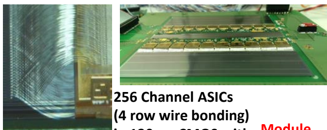
Module with on-board DC-DC converter
