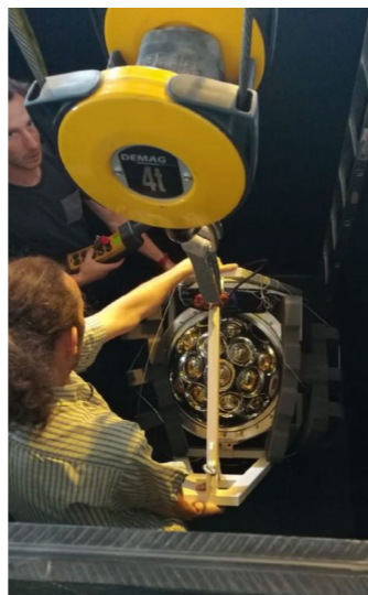
mPMT in Memphyno water tank in France
