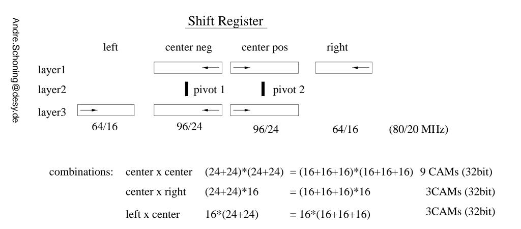
15 CAMS for each pivot element makes 30 CAMs in total
